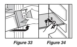
• **Removing drawers (Figure 33)**: Pull forward until the drawer stops and lift out.
